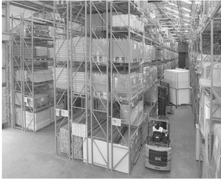
FIGURE 10.3 Double-deep racking (courtesy of Redirack)
