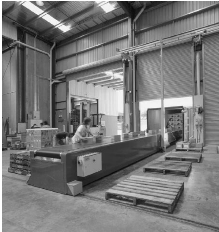
FIGURE 3.8 Boom conveyor unloading cartons (courtesy of Best Conveyors)
