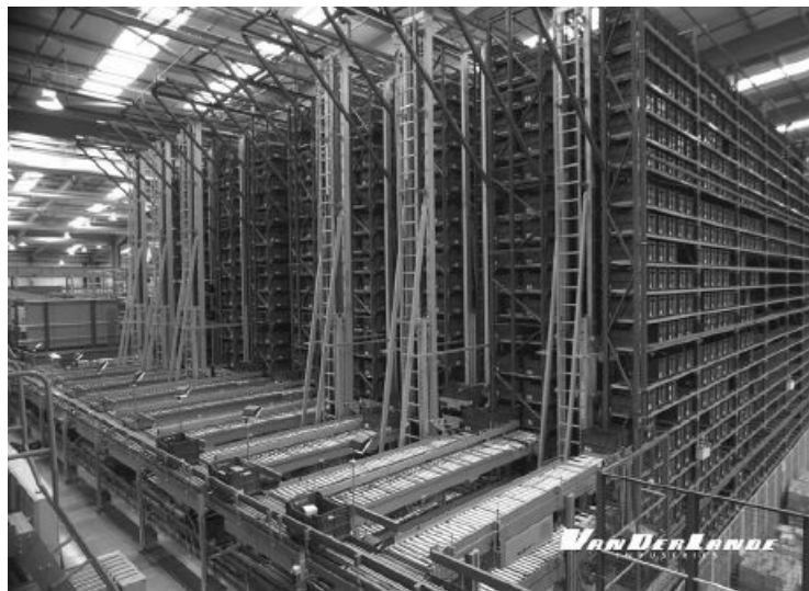
FIGURE 5.3 Mini-load system (courtesy of Vanderlande)
