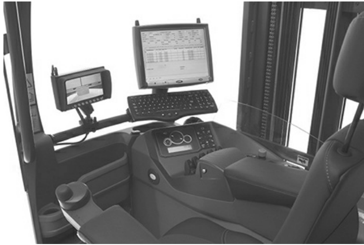
FIGURE 10.19 Internal view of computerized forklift truck (courtesy of Atlet)
