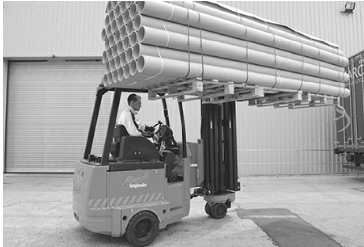
FIGURE 10.30 Articulated forklift truck with sideloading attachment (courtesy of Bendi)
